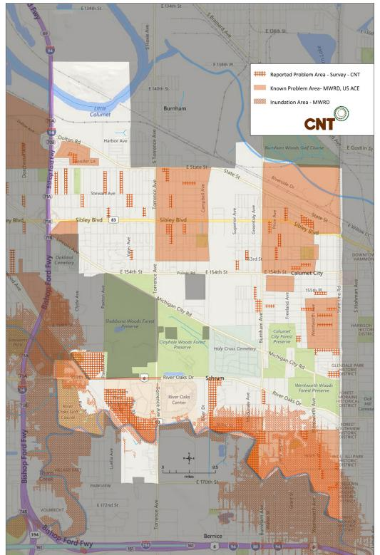
4) **Flat topography:** most stormwater is directed via gravity, so Calumet City's flat streets create challenges for moving the water out of neighborhoods.
